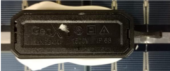
Junction Box closed view
