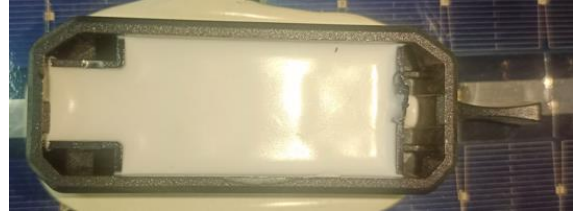
Junction Box opened view
